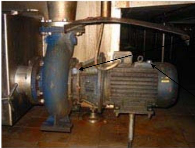
Placement of measurement pads on a machine
